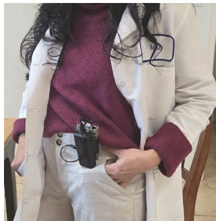
Figure 1: The MDwAIstScheduler system, designed to be worn on the belt and hidden beneath a lab coat during patient encounters.
